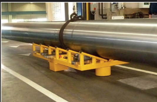
Remote-controlled trolley designed for 20 tons to transport high-quality drums
