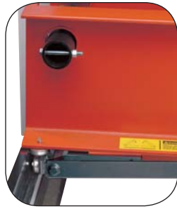
Bearings make bed positioning smooth and easy.
